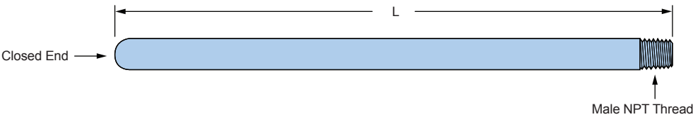
Style B: Pipe Type Protecting Tube with Mounting Bushing
